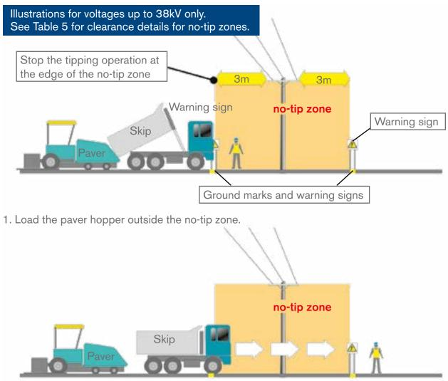
2. Fully lower the skip on the tipper truck, and any other elevated plant, such as a planer. before passing through the no-tip zone.
