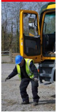
Correct method for exiting a vehicle when there is a risk of fire or other hazard
