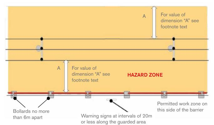
Dimension A = Minimum distance of **6m** for LV, 10kV, 20kV and 38kV Dimension A = Minimum of **10m** for 110kV 220kV, 400kV (and other voltages in this range)
