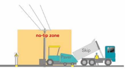
3. Continue normal operation when the tipper truck or other elevated plant is completely clear of the no-tip zone.
