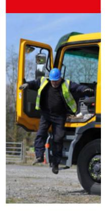
Shuffle away from the vehicle. Take half steps only or hop with both feet together to minimise the possibility of electric shock
